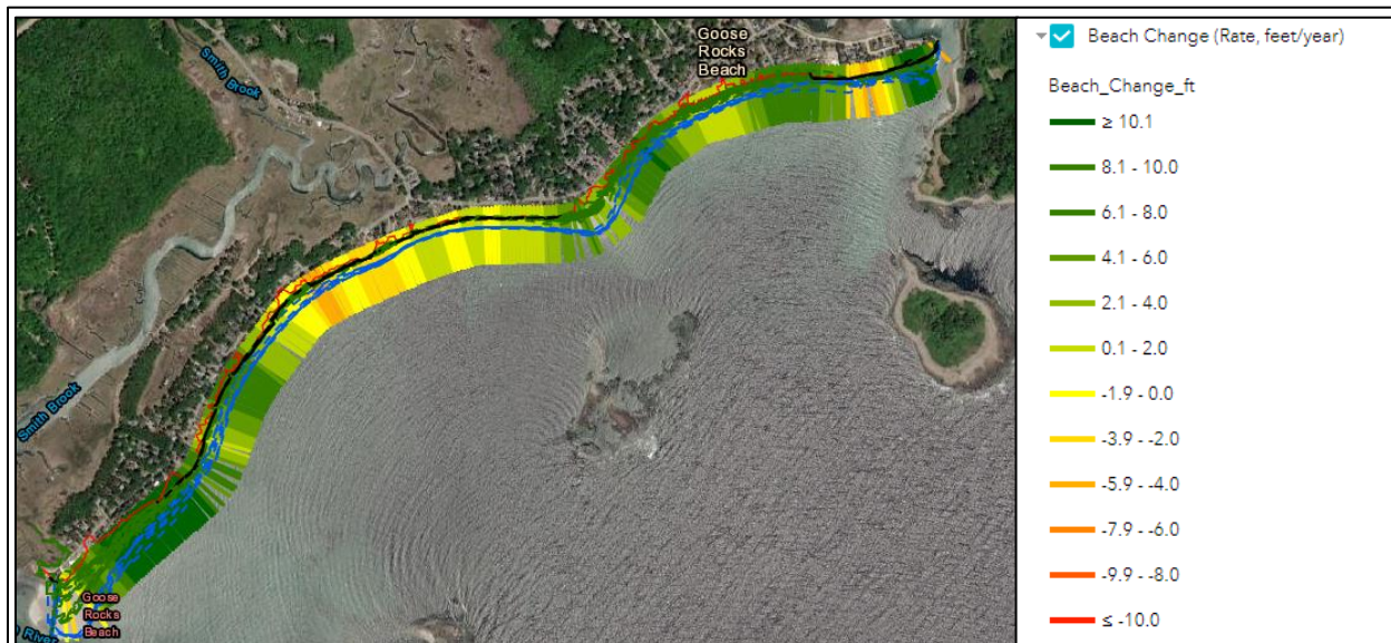
Map 15. Mapped shoreline change along Goose Rocks Beach. This map shows the rate of beach change, in feet per year, from data collected from 2016 through 2020. A positive value (green lines) represents a rate of beach growth, while a negative value (yellow/orange/red lines) represents a rate of beach loss. (Source: Maine Geological Survey. Maine Beach Mapping Program. Maine Beach Mapping viewer)
